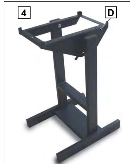
4. Add the cradle (D) by inserting the supports on the uprights
